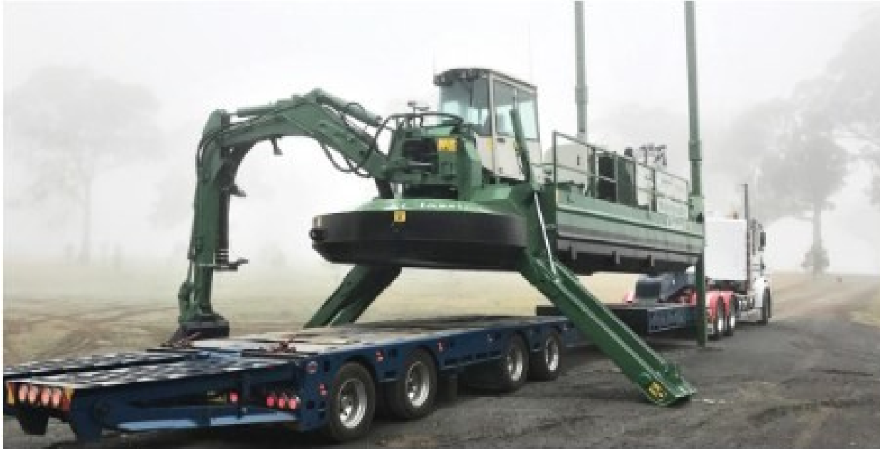
Highway-transportable: the machine walks on and off its own trailer.
